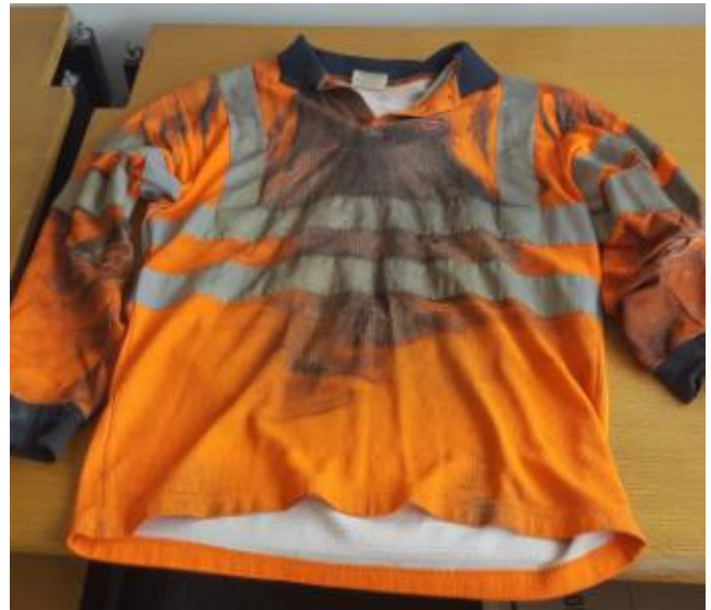
Flame and arc resistant shirt took the brunt of the flash. However the shirt was not damaged on the skin side. Neither were the upper arms.
