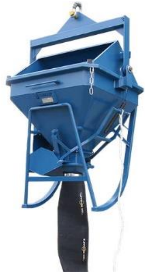
Type of skip being used at time of incident
