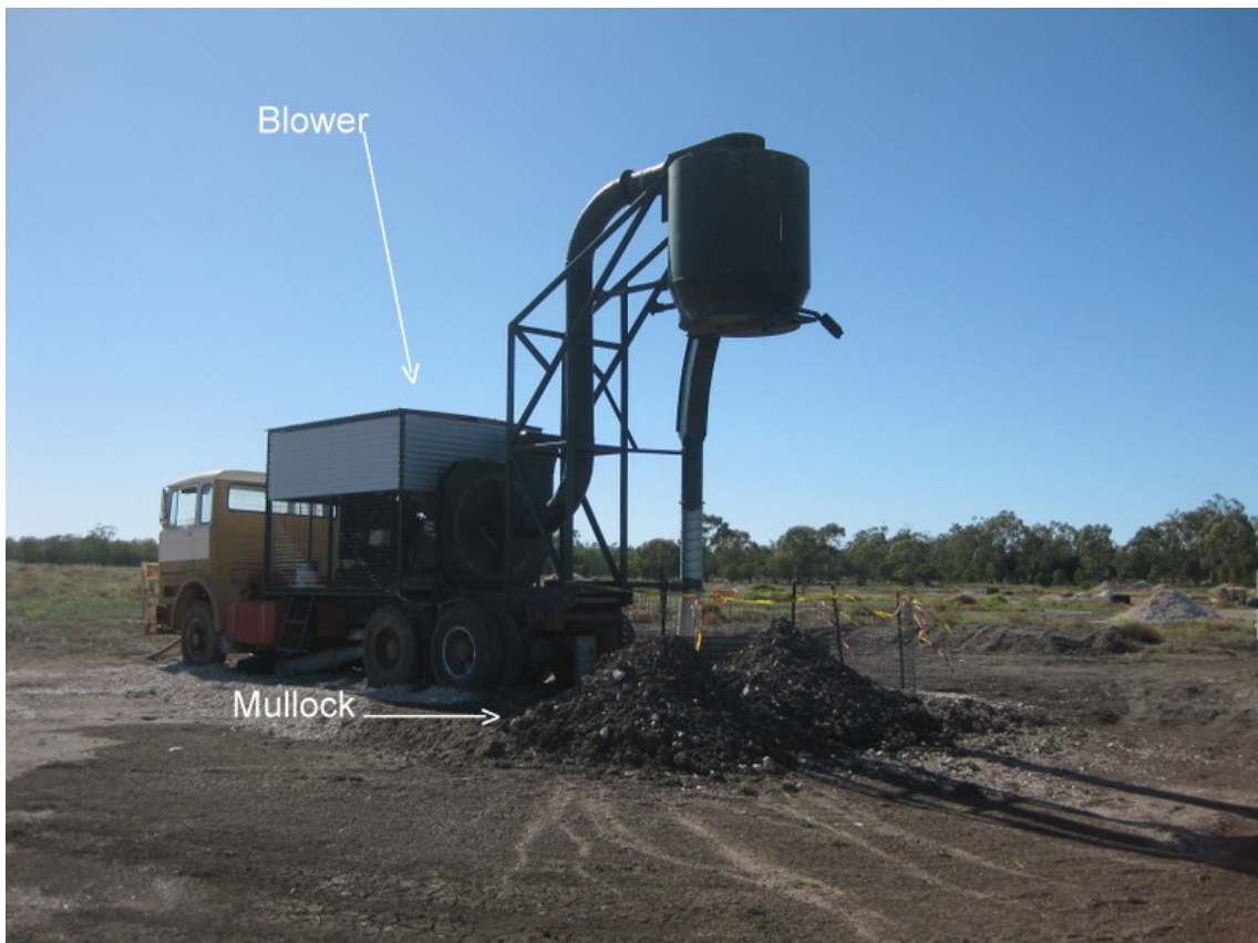
Figure 2: The truck mounted blower showing where the mullock fell. Photos by Mine Safety.
