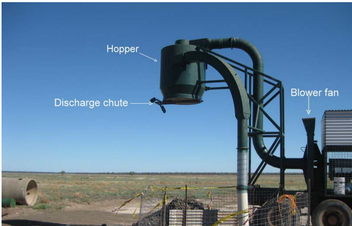
Figure 4: The hopper showing the discharge chute door. Photo by Mine Safety.
