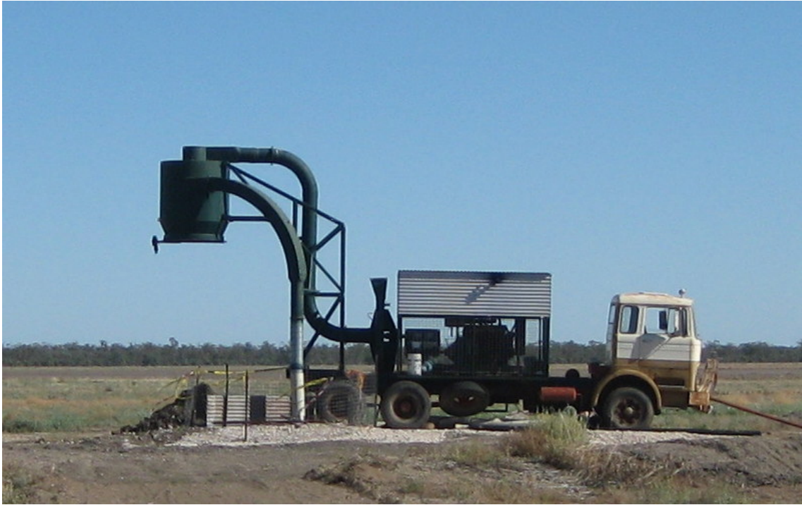
Figure 2: The truck mounted blower showing where the mullock fell. Photos by Mine Safety.
