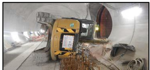
Overtuned excavator when being used as lifting equipment
