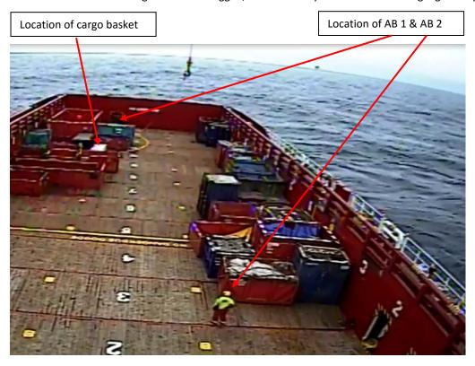
After a short time both AB's made their way back to the basket and cleared the lifting bridles. They then stood clear in a safe haven nearby while the crane took up the slack but once again the lifting bridle caught on the lid, this time buckling the lid exposing the cargo inside.
