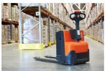
Electric pallets jacks are one of the most useful pieces of equipment within our company. If used correctly, they are highly efficient and can increase a picker's hourly case pick rate by 50%.
