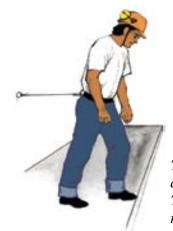
This is an example of a fall restraint system. The worker cannot fall off the edge.
