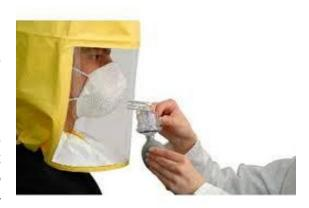
accepted fit tests. There are several methods with significantly different protocols for conducting **Quantitative fit testing** (QNFT). While the OSHA regulations and ANSI Z88.10 provide the procedures that must be used to conduct each of the accepted protocols, a general description of the most common methods used in the protocols are provided below for the convenience of the reader.
