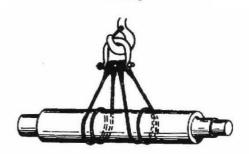
Double wrap sling grips the load and helps prevent it from slipping sideways
