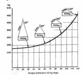
For all multi-leg chains the angle between the chain legs is critical – the greater the angle, the greater the safe working load of the chain to lift a given load. For example, to lift a load of 450kg using a two -leg chain, the SWL of each leg at an angle of 30 ° is 240kg, but if you increase the angle to 120°, the SWL increases to 450kg for each leg. This is shown in the accompanying diagram.
