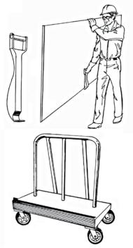
If the walking surface is level and hard, use a drywall cart.
