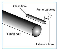
Relative sizes of a human hair, a glass fibre, an asbestos fibre, and fume particles. If there is enough room for a hair between the skin and the respirator, there is room for many contaminants to enter.
