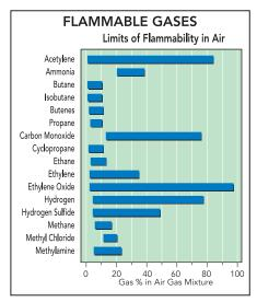
Figure 10 - Flammability Range of Gases
