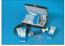
Model 8014KA Toxic Gas Detector Tube Sustem
