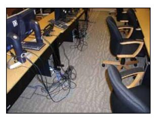
The cords for these computers protrude into an aisle and create a potential trip hazard.
