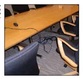
Providing an additional permanent electrical outlet closer to the computer to avoid running the cord across the aisle would be the best solution. When this is not feasible, it may be appropriate to use a cord strip protector when the aisle has minimal traffic.
