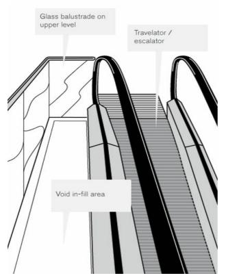
In-fill area made of plasterboard, which is not safe to stand on
