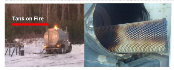
Visible Flame from Truck Tank Hatch
