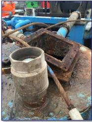
Estimated Weight of Steel Plate Potential Dropped Object was 2kg. From the DROP's calculator this could be fatal when falling from heights of 6.5 metres and above.
