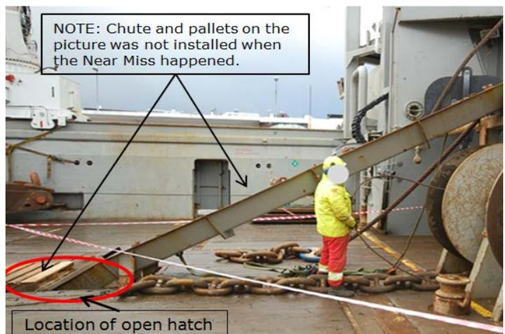
Pictures of a similar hatch opening into which the person walking backwards had fallen.
